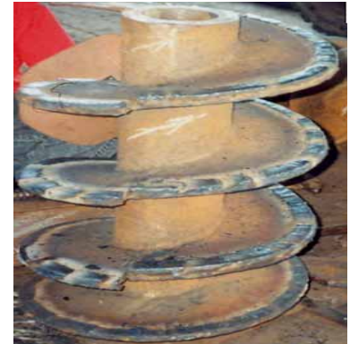
Protect screws for cement, sand, stone
