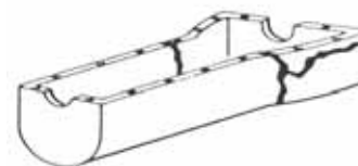
Weld oil impregnated cast iron (Oil sumps )
