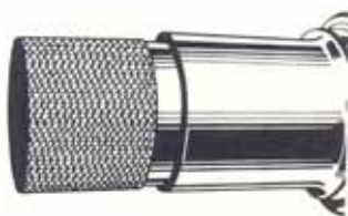
Rebuild worn shafts
