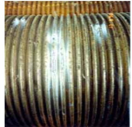
Cast iron roller repair with 420
