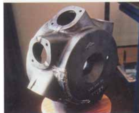
Repaired grey cast housing
